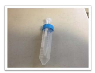
Place the 5cc centrifuge tube into the hole in the lid of the 10cc centrifuge tube
