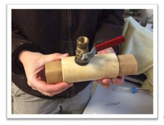
Place rubber tubing inside PVC and fold ends over the pipe
