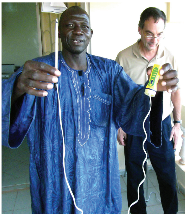
A simple light source can be constructed of locally available materials. Here a light source is constructed using an inexpensive flashlight (torch), lamp wire, and a drinking straw.
