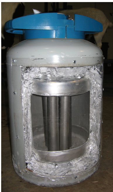
Cutout view of a liquid nitrogen semen storage tank showing insulation and canisters.
