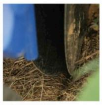
Double disk openers This tried and true system provides a uniform seed trench in various field conditions.
