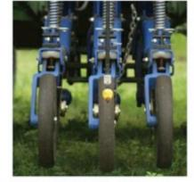
Packing wheels and herbicide nozzles These packing wheels ensure seed to soil contact and accurate planting depth adjustment for each of the three rows between each corn row.
