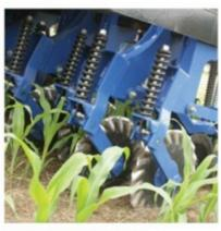
Coulters on planting units These coulters on each allow the interseeder to achieve good seed to soil contact in a wide range of soil and residue conditions.
