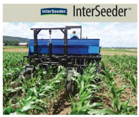
Three functions in a single, brilliantly engineered machine Cover Crop Planter • Liquid Fertilizer and Herbicide Applicator • No-Till Grain Drill
