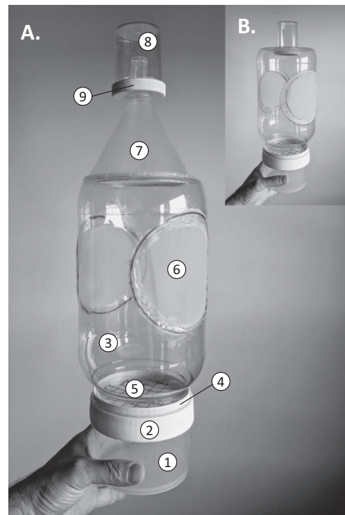
Fig. 1. (A) Components of the Lari-Leuco container: 1) a 500-ml round, straight-sided plastic jar, 2) screw cap to a 500-ml jar, 3) a 3.8-liter round plastic jar, 4) screw cap to a 3.8-liter jar, 5) a 10.5 cm diameter round piece of steel hardware cloth (1.27 cm opening), 6) a 12.5-cm diameter round piece of polyester mesh (435 \mu m opening), 7) a 12-cm diameter round plastic funnel, 8) a 118-ml round straight-sided plastic jar, 9) screw cap to a 118-ml jar. (B) Preliminary version of the container without the plastic funnel.
