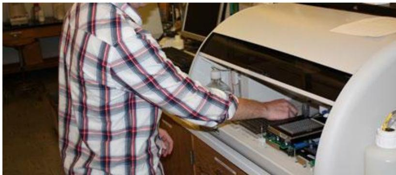
*The ChemWell multi-analyzer at the extension enology lab is like a big spectrophotometer and can perform any enzyme assay. A small winery can use a more standard spec and accomplish all of the same things, however.*
