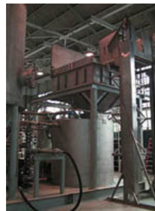
TDP pilot plant in Philadelphia, PA produces oil from turkey processing waste. Photo is courtesy of Changing World Technologies (CWT).
