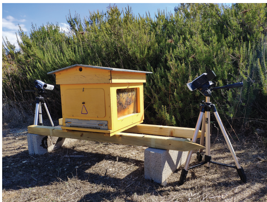
Photo 1 The whole-colony observation hive setup used to monitor behaviors of bees in varroa-infested vs. varroa-free colonies.
