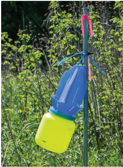
Photo 1 Blue Vane Trap, a type of insect trap that attracts and captures a wide variety of bees and other pollinating insects
