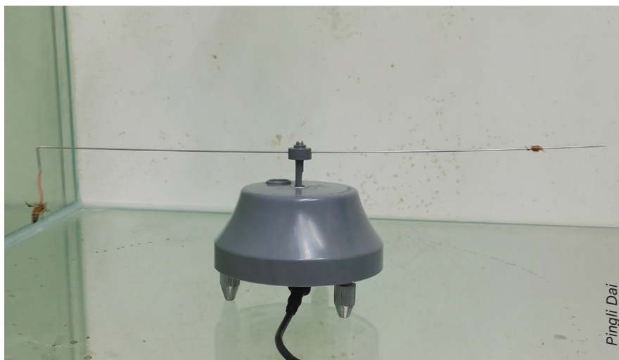
Photo 2. Flight mill used to test the flight ability of tethered forager bees
