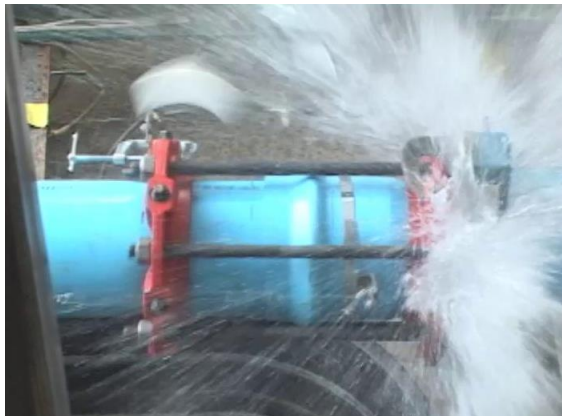
Figure 4.15. Joint Tension T2 – Pipe Rupture
