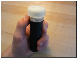
Figure 1: Our pressure-sensitive tangible self-report device for pain that can be embedded into serious toys in order to improve data capture from children
