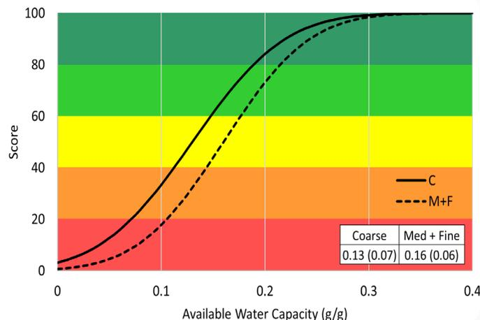
**FIGURE 3.** Available Water Capacity (AWC) scoring functions and upper value limits for Coarse (C), Medium (M) and Fine (F) textural classes. Mean and standard deviation (in parenthesis) for each class are provided. In this case more is better. Higher AWC scores indicate a greater capacity of the soil to store plant available water.
