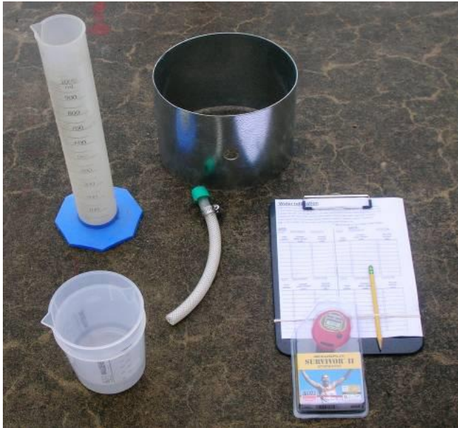
Fig. 2. Field infiltrability kit. These items fit nicely into a 5 gallon pail with a 2 pound hammer and a 4" x 4" x 12" wooden block
