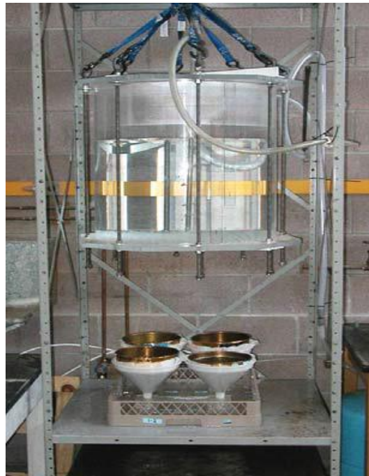
Figure 6. Extra large (60cm diameter) Cornell Sprinkle Infiltrometer drips on four 20cm sieves with soil samples simultaneously in the Cornell Soil Health Lab
