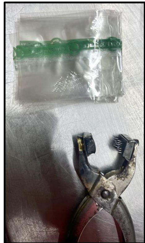
Image 2. Biodegradable cellophane packaging manually punctured with a perforator tool. (Image courtesy of Eileen Downs at Merle Maple)
