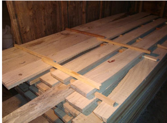
Figure 5. Lumber should be stickered immediately after sawing, ideally as the boards come off the mill. In door storage, as illustrated, is ideal if space is available.
