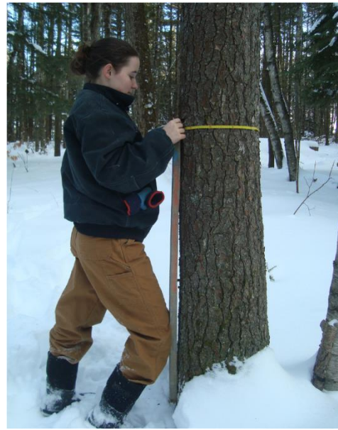
Figure 4. Repeated accurate diameter measurement of this white pine is simplified by a nail at approximately 12 inches above ground and a 3.5 ft stick.
