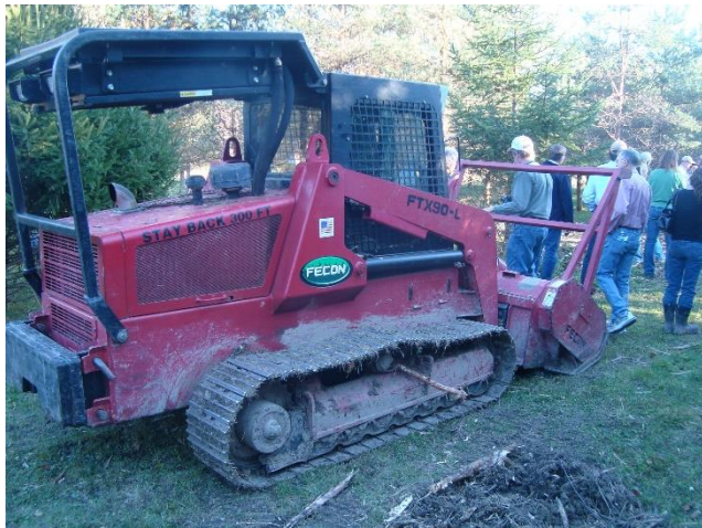
Figure 7. Fecon mower heads can be used for broadcast mechanical, and to some extent selective mechanical treatments of large stems or areas otherwise difficult to access.
