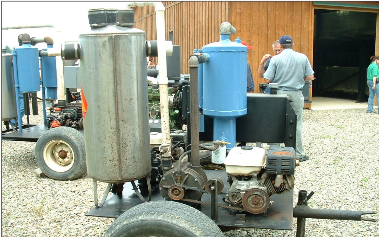
Portable vacuum pump and gas motor set up for remote locations away from electric
