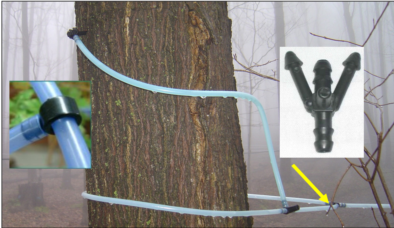
(left) End ring commonly used on the end tree, (middle) typical double tee method, (right) dead end loop fitting with straight through drop line to lateral line connection
