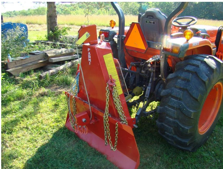
Figure 3. Special attachments for ATV and tractors, shown here with a winch, increase safety and productivity. Care is needed if these types of machines are used for small scale logging.
