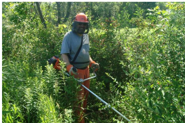
Figure 5. Brush saws are effective tools for vegetation management. The shoulder strap provides a barrier for kickback that would injure the operator. Safety equipment is still necessary.
