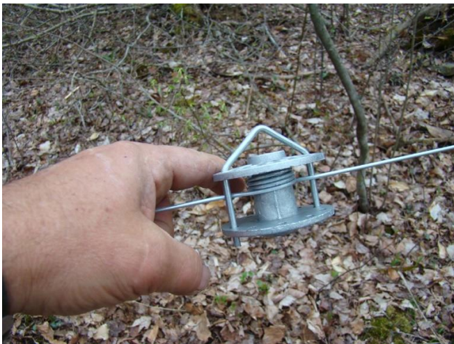
Figure 14. In-line tensioners used to tighten the 12 gauge wire.
