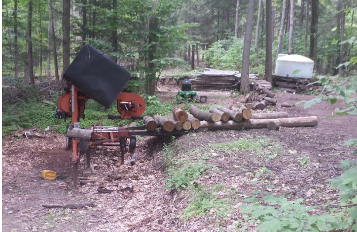
Figure 4. Advance planning will allow arranging logs in a manner to more easily load the sawmill. Creating a cut bank or using a gentle slope makes easy work of loading logs if the sawmill lack hydraulics logging.
