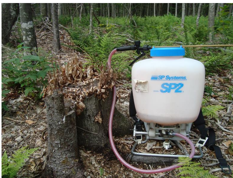
Figure 4. Backpack sprayers are inexpensive and handy tools for applying foliar, basal bark, and cut-stump applications of herbicide. Several brands of sprayers are available. Knowing the correct mixing concentration will reduce waste, minimize unnecessary applications of herbicides, and improve the success of the treatment. The sprayer brand pictured holds approximately 3 gallons, the V_2 used in Formula 2.
