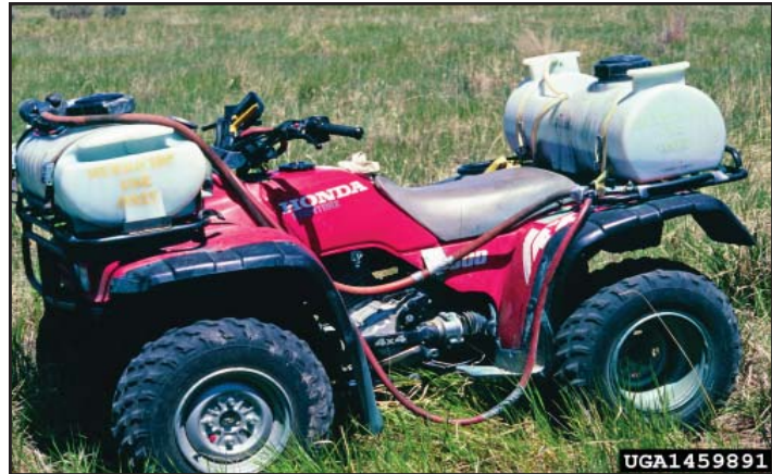
Herbicides can be sprayed from ATVs with a few extra attachments. Spot treatments, at the specific planting location, will reduce the amount of herbicide needed to control vegetation. Photo – S. Dewey, Utah State University, bogwood.org
