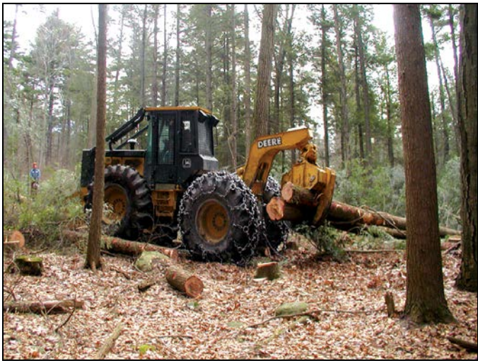
Because most roots are near the soil surface, they are susceptible to damage from heavy equipment, especially when soils are wet.
