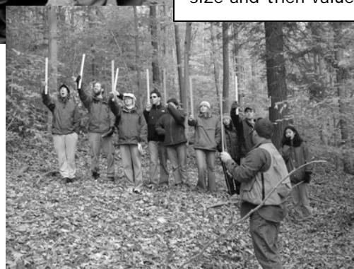
Foresters and forest owners can use a scale stick to estimate the size and then value of a tree.
