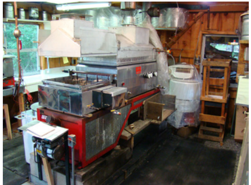
Figure 1. Modern maple production is still just boiling sap into syrup but involves an often involved process of highly engineered vacuum pumps, reverse osmosis, high efficiency evaporators and storage in controlled environments.
