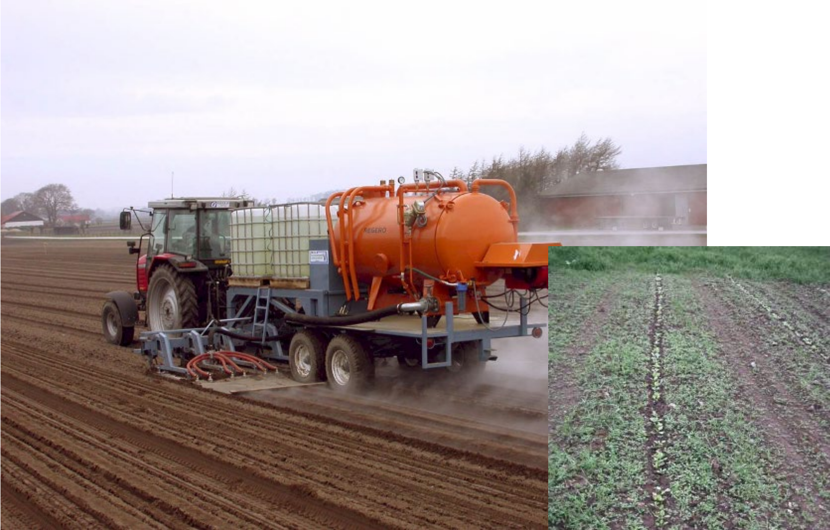
Left: band-steamer. Right: sugar beets emerging in row cleaned by pre-emergence band-steaming.
