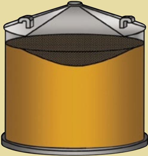
Figure 6. Grain spoilage caused by moisture migration.
