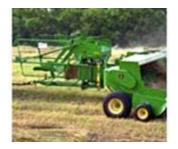
Finally, if the small square baler is equipped with a bale thrower (sometimes called a "bale ejector"), then the bales are tossed directly into a steel- or wooden-sided wagon, essentially baling and collecting the hay with one pass through the field. This reduces hay handling labor in the field because the thrower tosses the bale directly into the trailing wagon. (See picture at left of a small square baler equipped with a bale ejector.)
