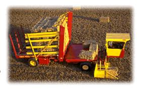
bales is required with this system. Examples of bale wagons that are built by New Holland can be found at: <a href="http://www.newholland.com/na/Products/BaleWag.html">http://www.newholland.com/na/Products/BaleWag.html</a>. The bale wagon operator will be constantly operating controls and maneuvering the bale wagon to load or pick up bales from the field.
