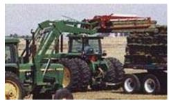
with a grabber, loading a group of bales on a wagon.) With a system like this, small square bales are easily handled in the field and during transport/storage without having to manually lift the bales. Accessibility issues are again focused on the operator requirements for access to and operation of the skid steer or tractor with loader.
