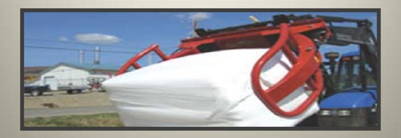
Use only front or rear tractor mounted specialized handling equipment to transport wrapped bales.
