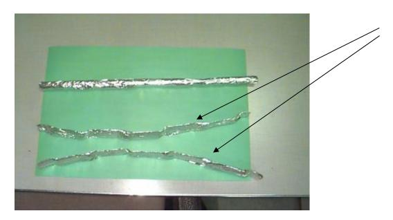
6. The rolls will crush the foil rolls and the minimum roll clearance can be determined by using a digital or dial caliper to measure the thickness of the foil roll. A low-cost digital caliper (~\$40) can be found at Techni-Tool (Part No. 575GA103, 1-800-832-4866). Take several measurements of the thickness along the length of each foil roll and determine an overall average. The measurement should be taken where the "crimp" or smallest clearance occurs as noted in the above figure.
