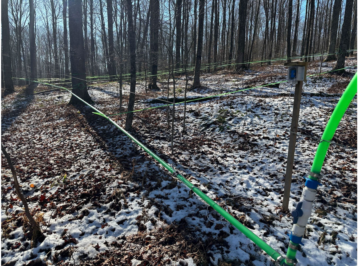
Sensor monitors sap temperature in a collection system demonstrating strategies for sugaring in a warming climate in the Arnot Teaching and Research Forest
