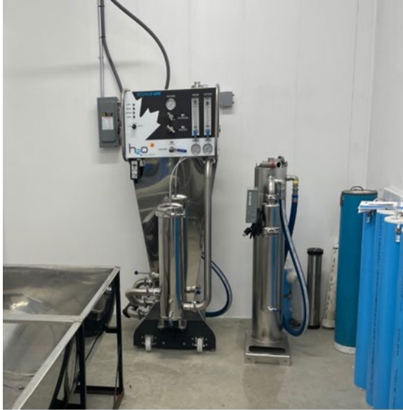
Experimental ultrafiltration unit at Arnot Maple Lab removes microbial bodies from sap. Prefiltered concentrate on left, filtered concentrate on right
