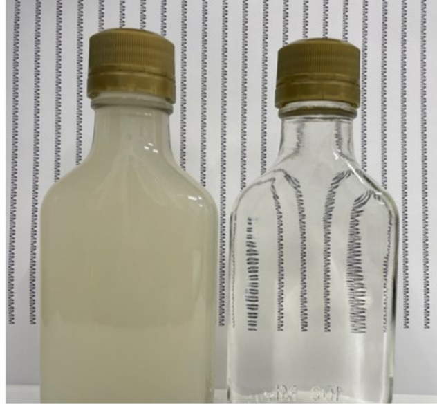
Experimental ultrafiltration unit at Arnot Maple Lab removes microbial bodies from sap. Prefiltered concentrate on left, filtered concentrate on right
