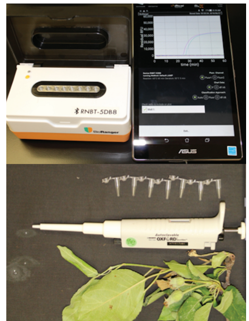
Figure 4. BioRanger device, an android Tablet on top, infected test branch, pipette and PCR tubes below).
