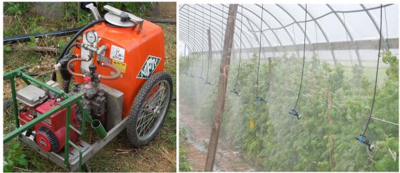
remaining in the tubing after spraying was finished, a length of hose attached to a valve on the PVC manifold drained off much of the contents of the supply lines into a container; this was used to fill a backpack sprayer for treating check rows in an adjacent HT planting not fitted with the fixed spray system.
