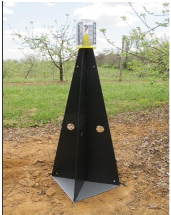
Pyramid trap (AgBio) used in multi-state trials to evaluate BMSB pheromone lures.
