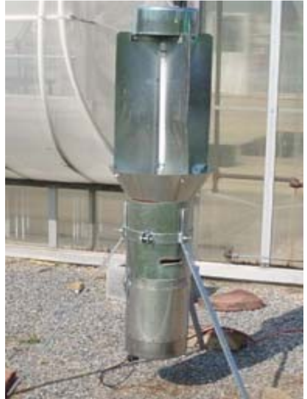
This black light trap stands guard against fruit and vegetable pests, including the brown marmorated stink bug, in a network of about 70 similar traps in New Jersey. Source: G. Hamilton, Rutgers University
